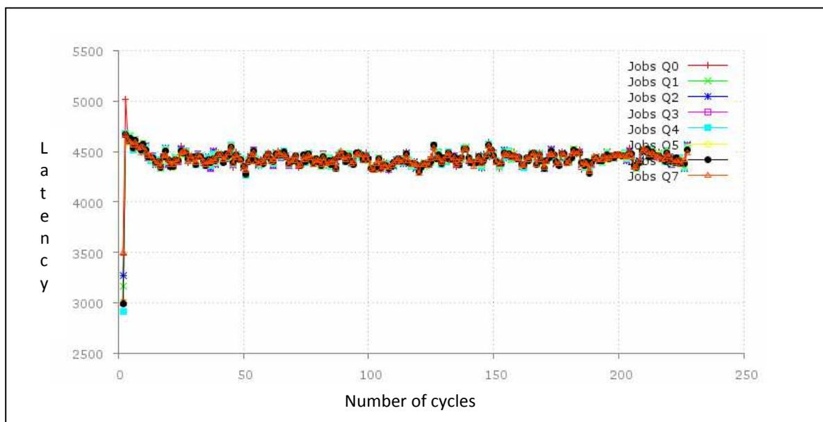
Figure 6.13-1 Latency for each time a packet is dequeued then a new packet is enqueued in the same queue. Average packet weight 100, minimum queue weight 300, maximum queue weight 1000.
