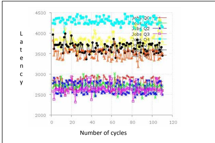
Figure 6.8-1 Latency for packets with minimum queue weight 300, maximum queue weight 1000, average packet weight 100 for Q0-Q3, average packet weight 50 for Q4-Q7.
