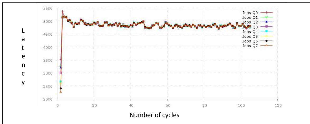
Figure 6.14-1 Latency for each time a packet is dequeued then a new packet is enqueued in the same queue. Average packet weight 50, minimum queue weight 300, maximum queue weight 1000
