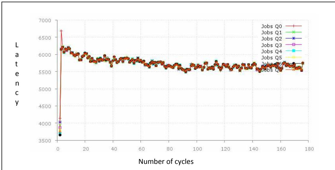
Figure 6.15-1 Latency for each time a packet is dequeued then a new packet is enqueued in the same queue. Average packet weight 100, minimum queue weight 650, maximum queue weight 1000.
