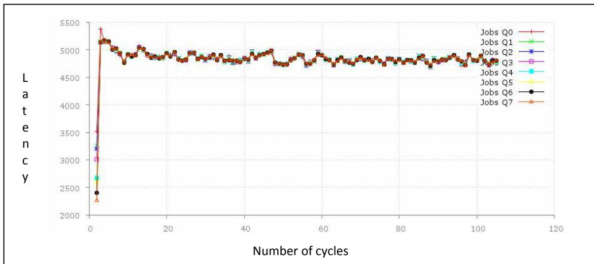
Figure 6.16-1 Latency for each time a packet is dequeued then a new packet is enqueued in the same queue. Average packet weight 50, minimum queue weight 650, maximum queue weight 1000.
