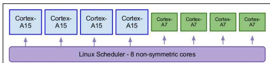
Figure 3.1-3 heterogeneous multi-processing (MP)[6]
