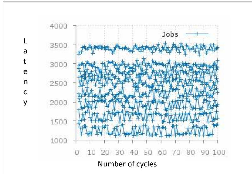
Figure 6.2-1 Latency for as many packets as can be served in a cycle average packet weight 50, min queue weight 300, max queue weight 1000.
