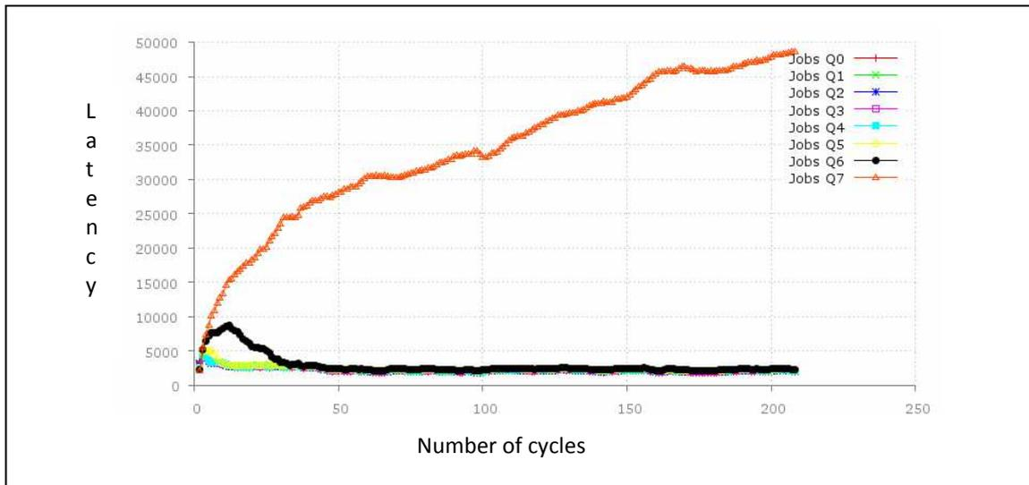
Figure 6.12-1 1 Latency for average packet weight 50, insert 3 new packets every 800 quanta, minimum queue weight 300, maximum queue weight 1000.
