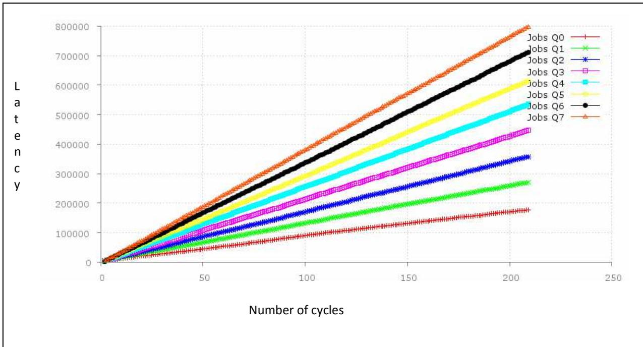
Figure 6.9-1 Latency for average packet weight 100, insert 3 new packets every 800 quanta, minimum queue weight 300, maximum queue weight 1000.
