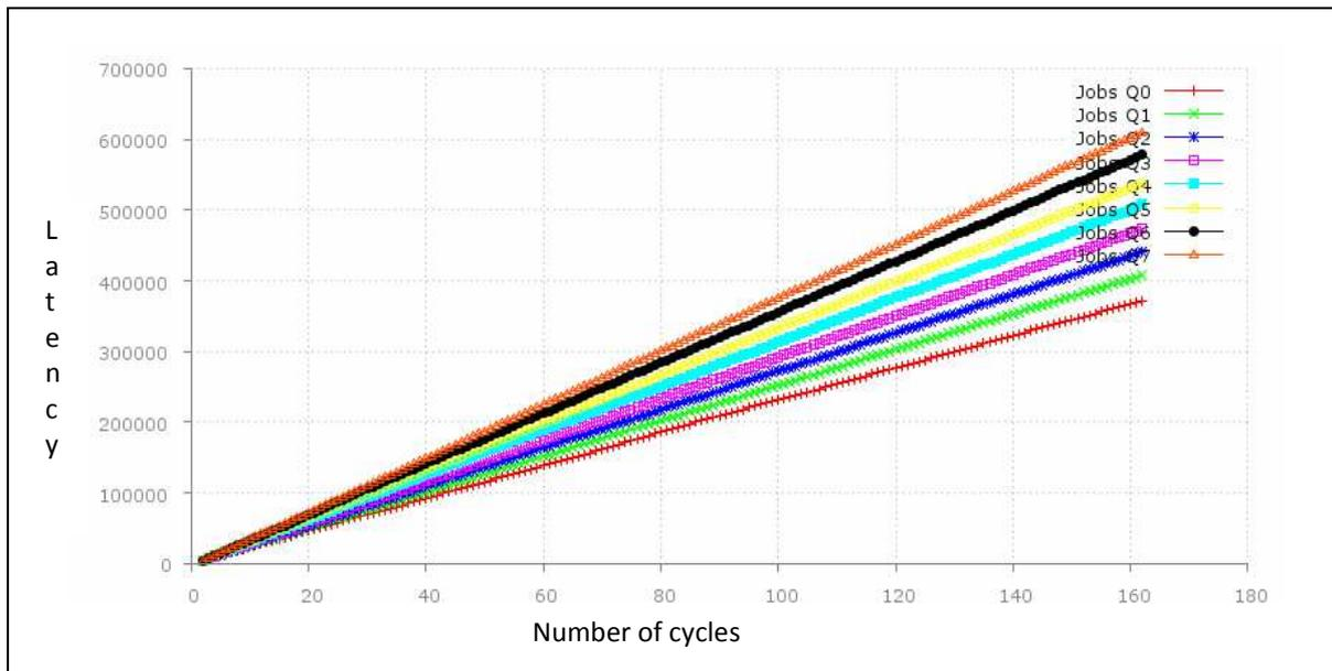
Figure 6.10-1 Latency for average packet weight 100, insert 3 new packets every 800 quanta, minimum queue weight 650, maximum queue weight 1000.
