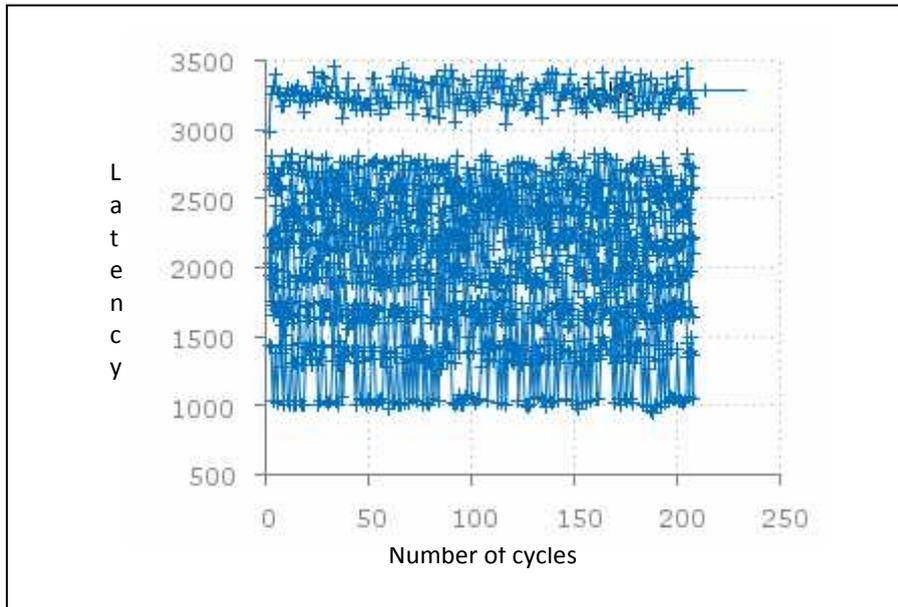
Figure 6.1-1 Latency for as many packets as can be served in a cycle average packet weight 100, min queue weight 300, max queue weight 1000.
