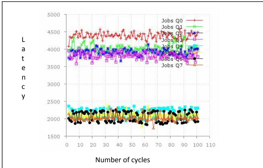
Figure 6.7-1 Latency for packets with minimum queue weight 300, maximum queue weight 1000, average packet weight 50 for Q0-Q3, average packet weight 100 for Q4-Q7.
